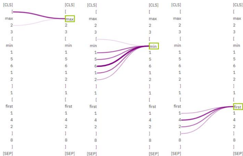
FIGURE 3.4: Figure shows that operators inside each sub-sequence are attended by their tokens in layer 6.
